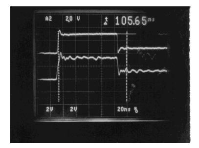
Top signal = top of the extender; bottom signal at the slot (ringing at the bottom signal is due to a longer scope probe)
