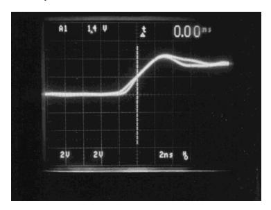
One channel at source and other channel at top of the extender
